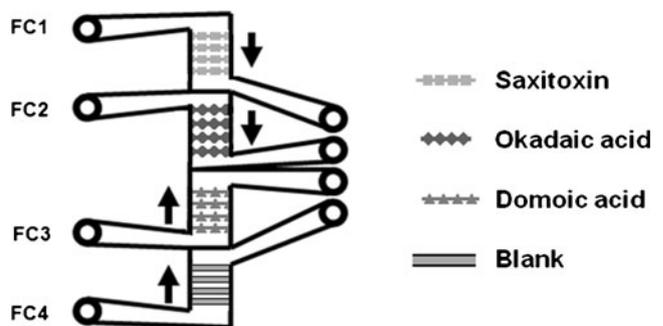
**Fig. 1** Layout and spotting of the four flow cells (FC) for the prototype multiplex SPR biosensor chip. Four spots of each toxin was spotted in each FC (leaving FC4 as a blank to be used as a control to ensure immobilisation was successful) allowing samples to be analysed in quadruplicate. Arrows show the flow of samples across the individual flow cells and the inlets/outlets for each flow cell being separate from each other
