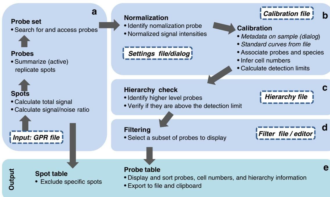
**Fig. 3** Structure of GPR-Analyzer with major components: internal representations of the GPR file (a), normalization and calibration (b), hierarchy checking (c), filtering (d), and output (e). *Italics* indicate user/file input
