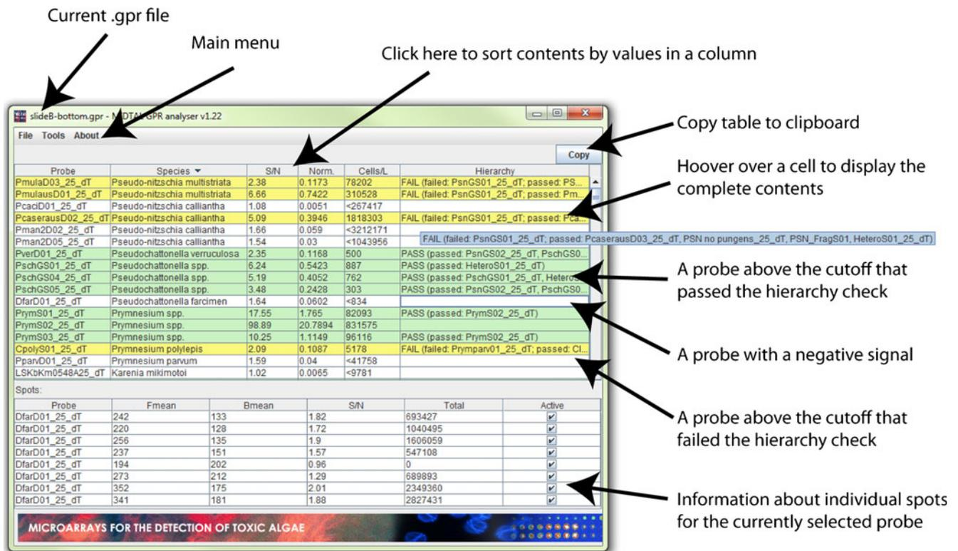
**Fig. 4** Screenshot of the main window of GPR-Analyser displaying a sample GPR file. Green color-coding indicates probes for species likely to be present, yellow potential false-positives based on hierarchical or parallel probes, and white negative probes
